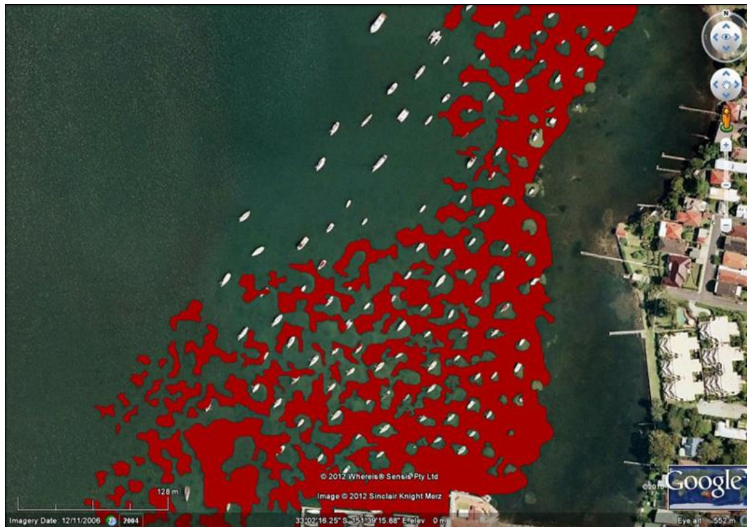
Figure 2.10 – Aerial image showing scouring of Posidonia australis beds in Belmont Bay as a result of traditional block and tackle or swing moorings. Source: Wright et al. , (2013)
